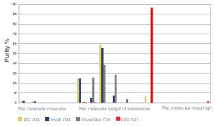
A low relative molecular mass and mixtures of various substances in the oil interfere with the performance of diffusion pumps. LVO 521 contains a very high-purity of a special silicone to help you to get the best performance from your pump.
